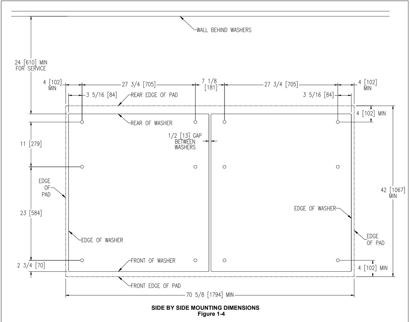
*2.7.23 T-900/950 Machine Side By Side Mounting Detail*
