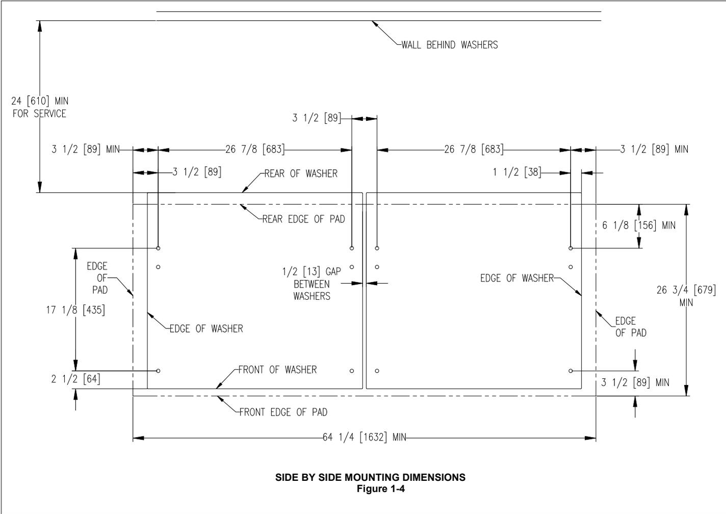
*2.7.8 T-400 Machine Side By Side Mounting Detail*
