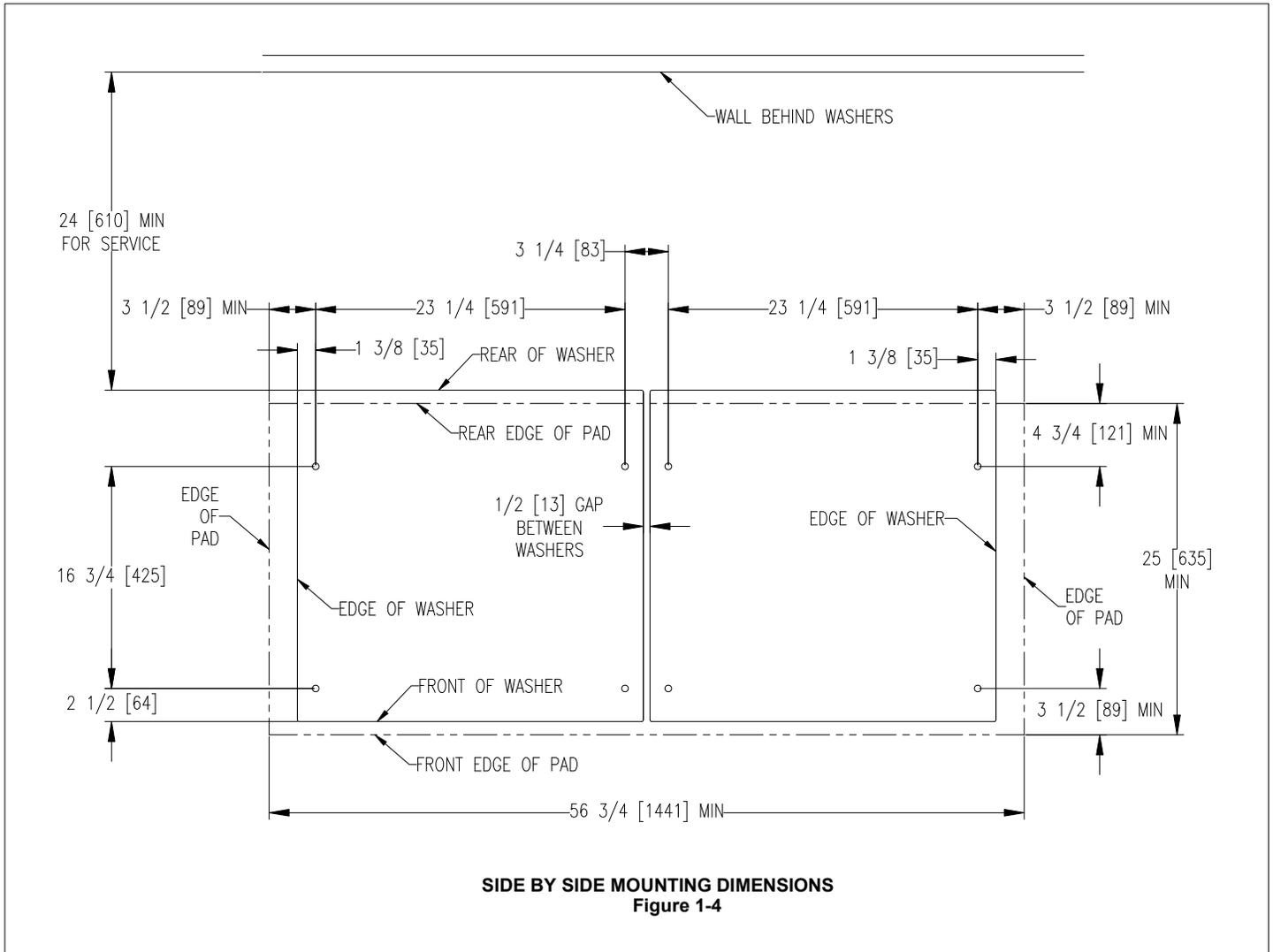
*2.7.2 T-300 Machine Side By Side Mounting Detail*
