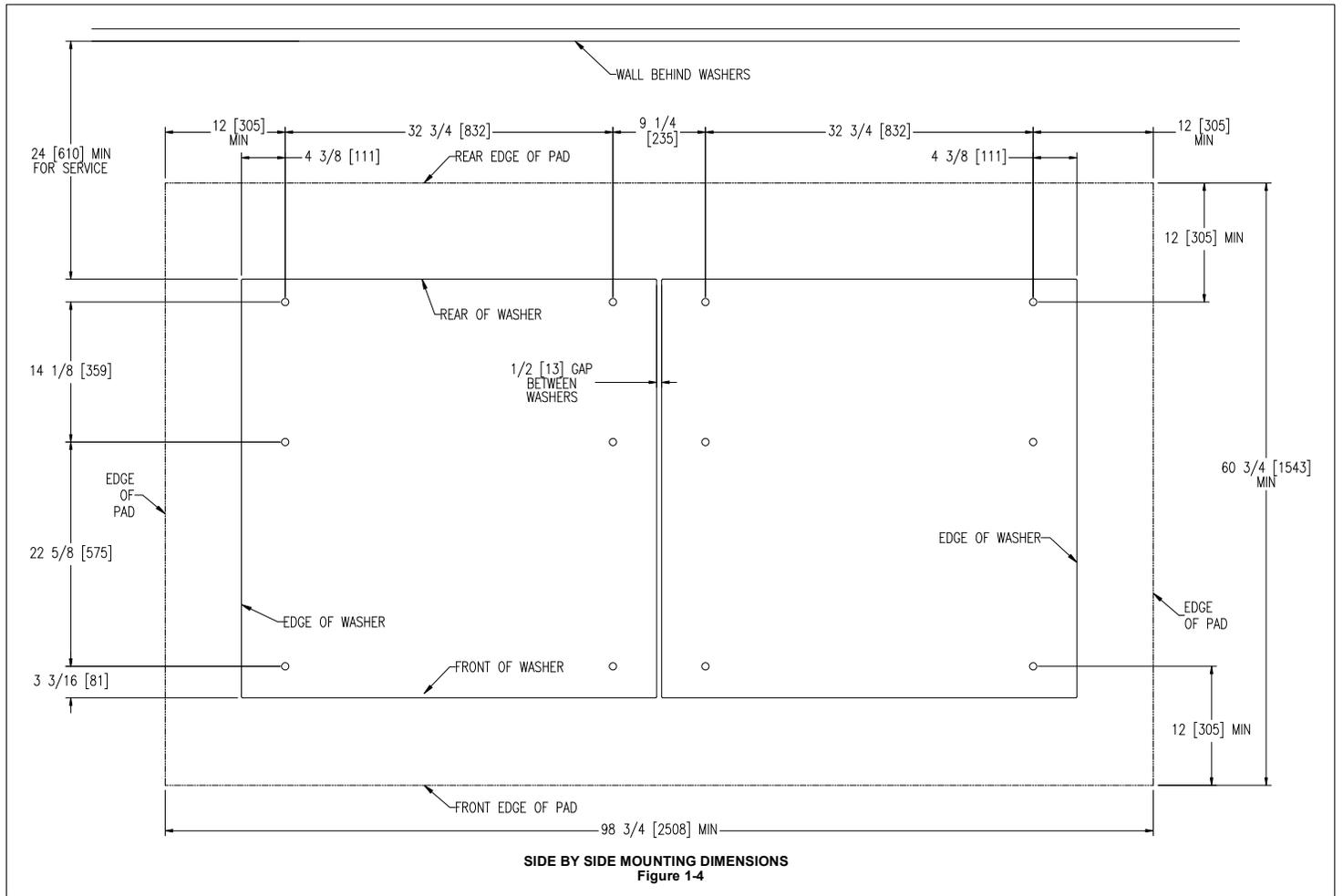
*2.7.29 T-1450 Machine Side By Side Mounting Detail*
