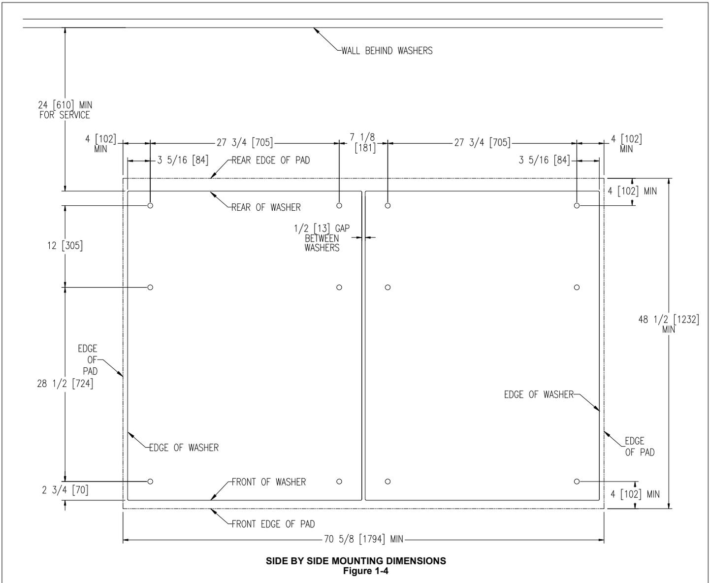
*2.7.26 T-1200 Machine Side By Side Mounting Detail*
