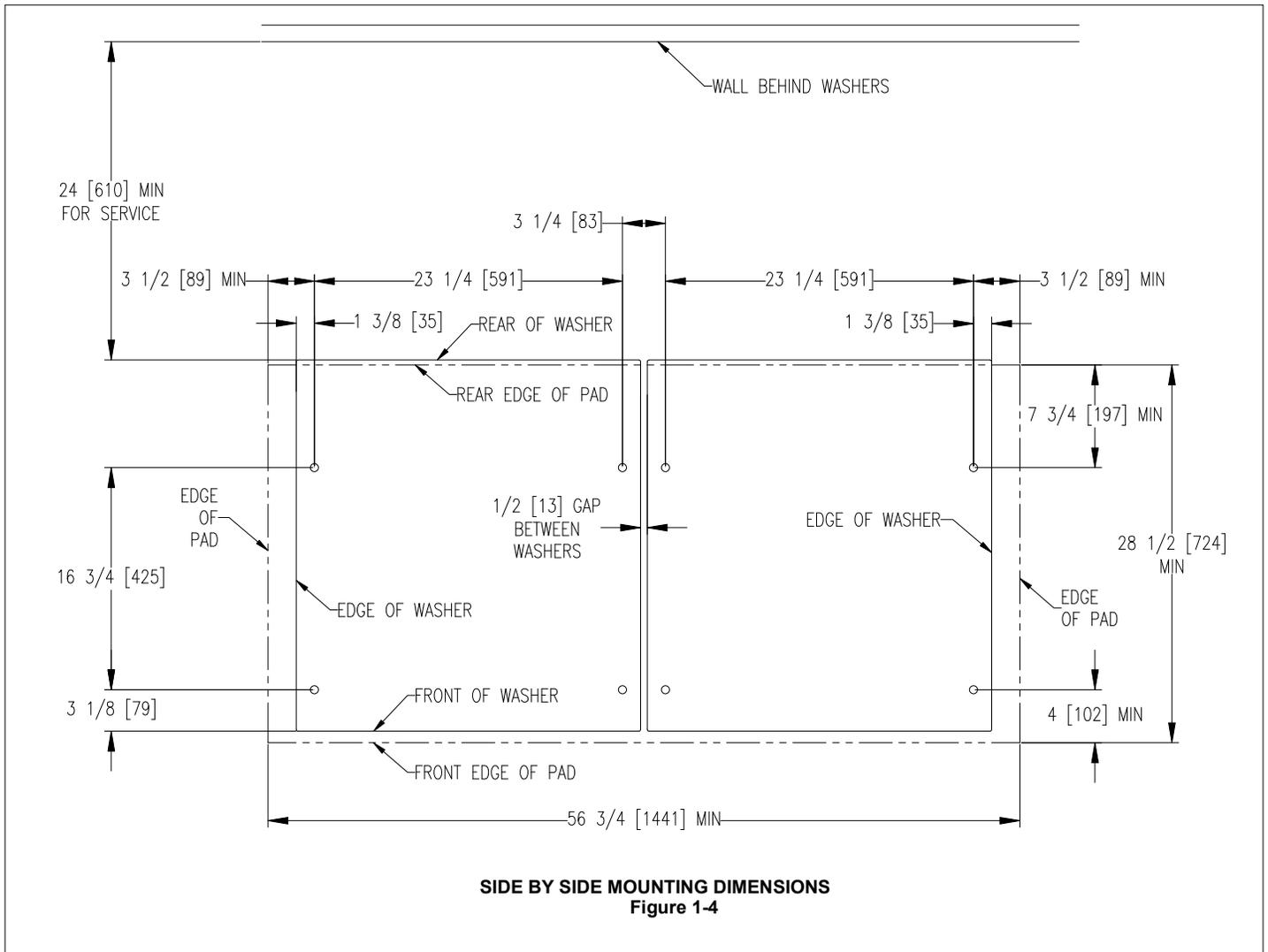
*2.7.5 T-350 Machine Side By Side Mounting Detail*
