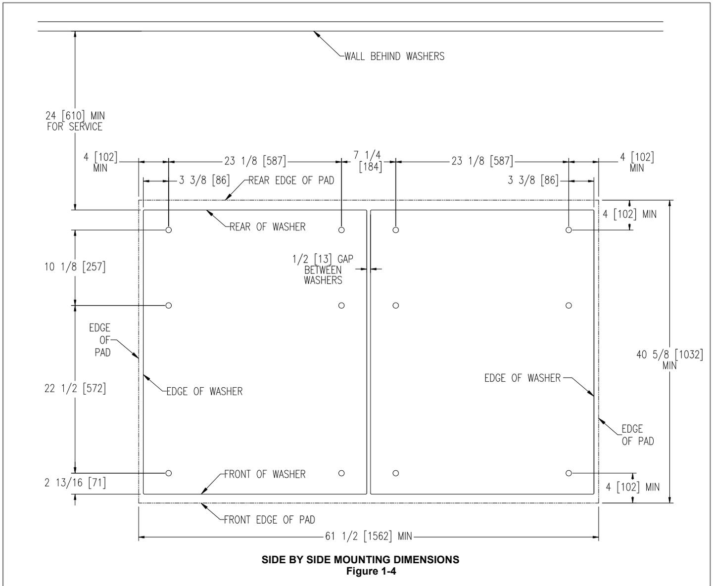
*2.7.17 T-650 Machine Side By Side Mounting Detail*
