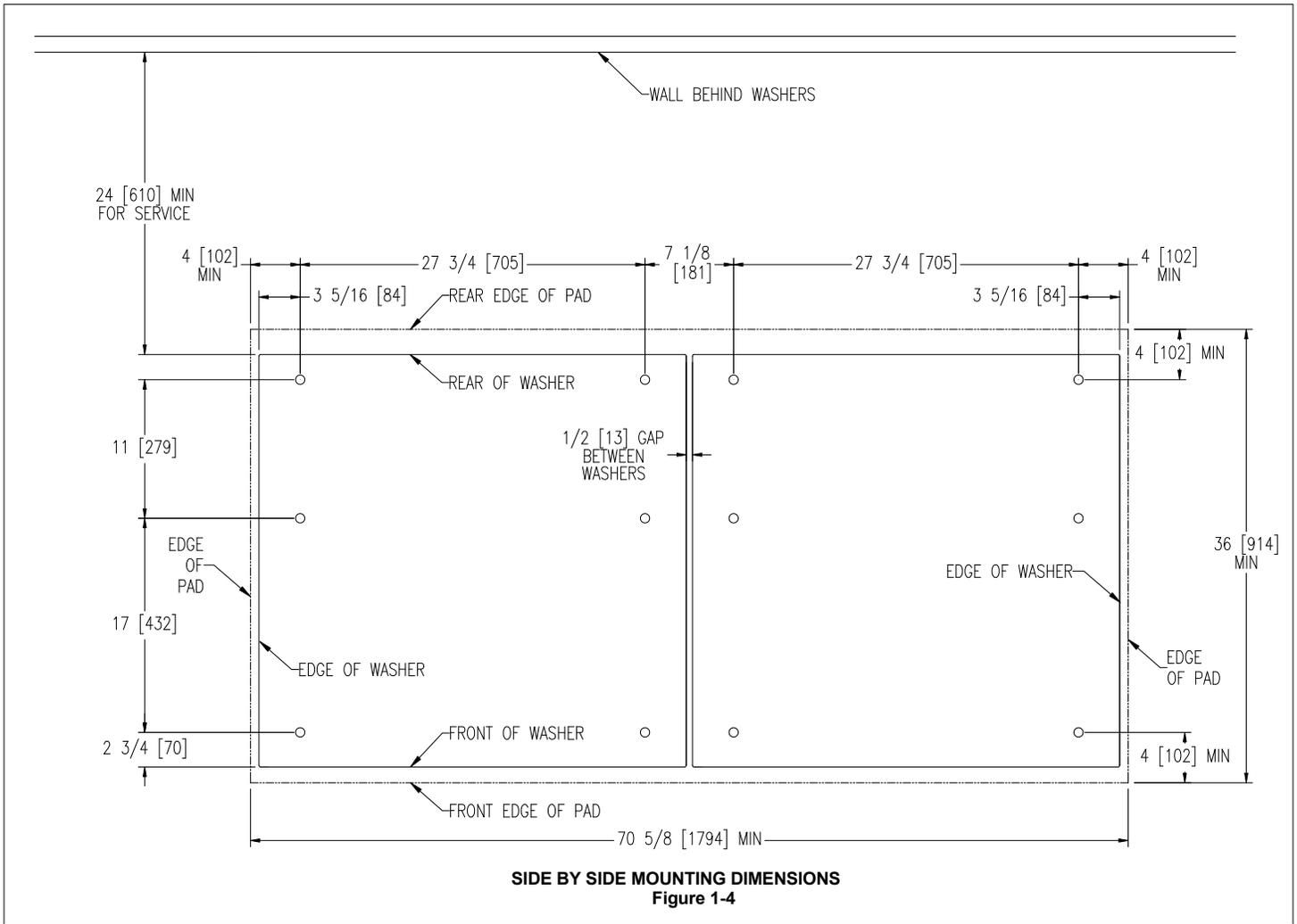
*2.7.20 T-750 Machine Side By Side Mounting Detail*
