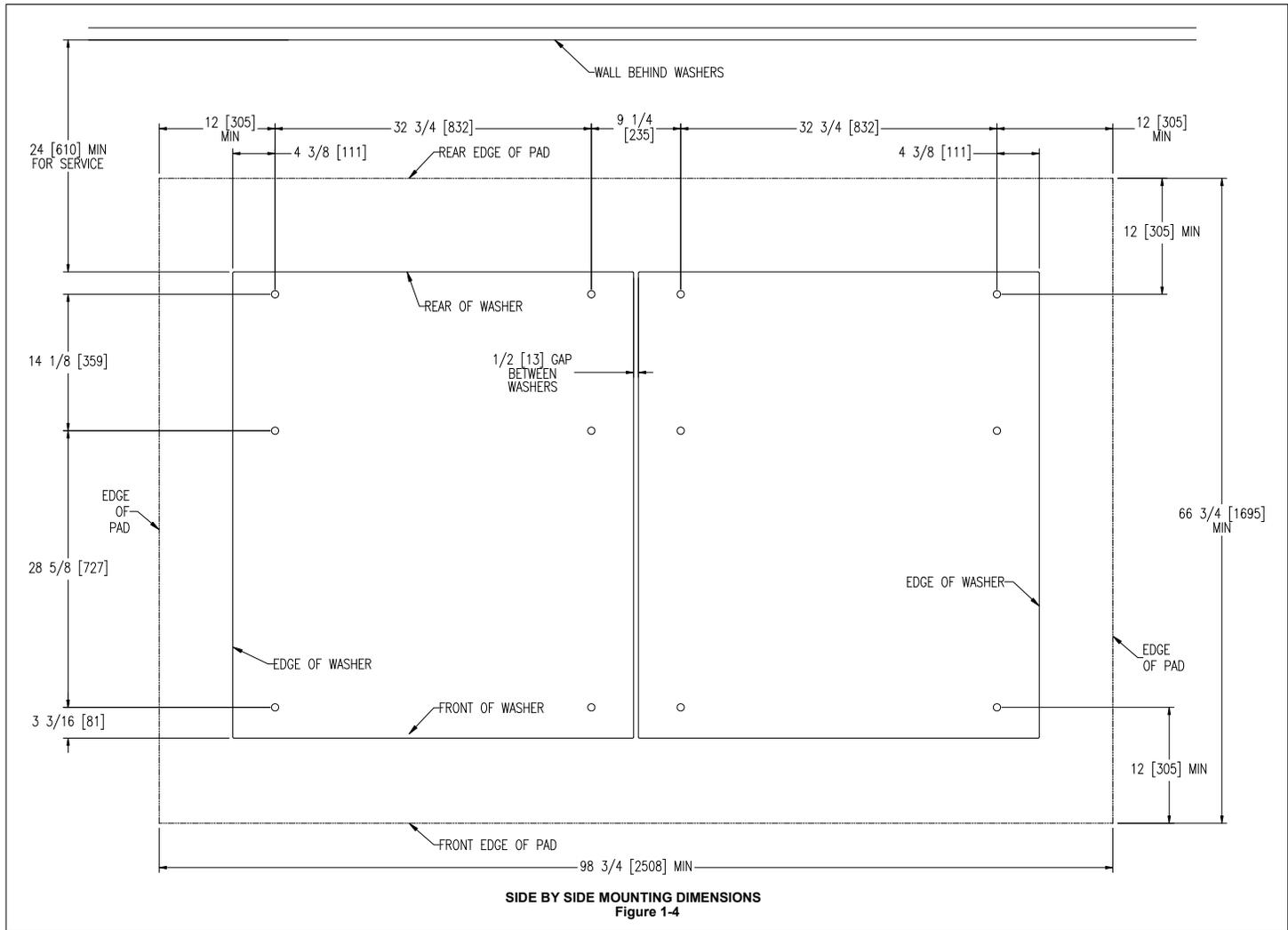
*2.7.32 T-1800 Machine Side By Side Mounting Detail*
