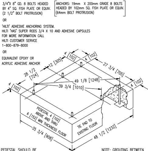
PEDESTAL SHOULD BE 4,000 PSI [28 MPa] MIN CONCRETE REINFORCED WITH MESH OR RODS.
