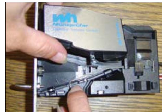
Open the flap of the coin selector.
