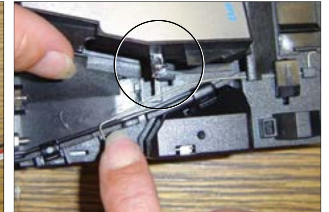
Move spring downwards to free the catch.
