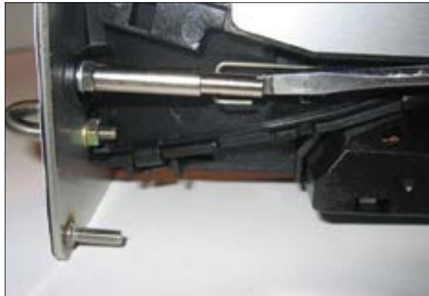
Once the bolt is fixed, please verify the position of the spring as indicated in the picture.
