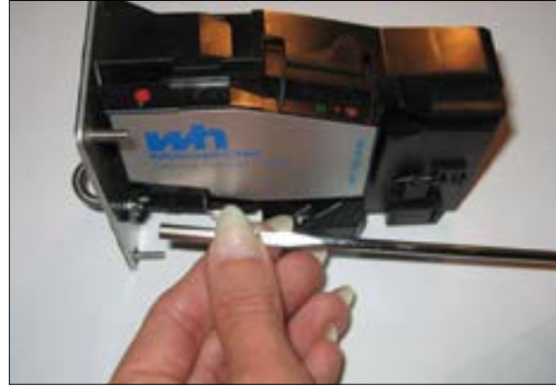
Screw the bolt onto the existing stud weld on top of the nut which fixes the reject bracket.
