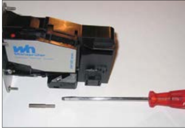
The bolt (part number 4036) should be mounted with the help of a screw driver.
